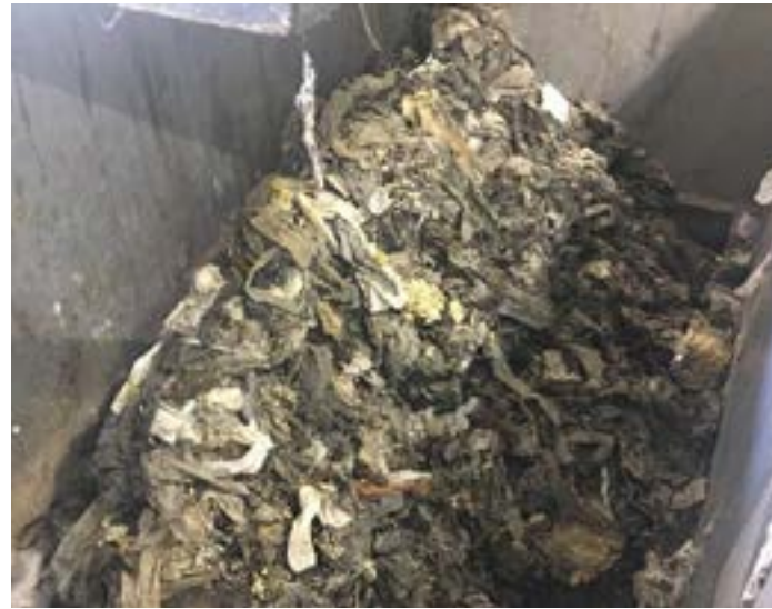
Used wipes collected in a disposal bin after being removed from a sewer in Macomb County MACOMB COUNTY PUBLIC WORKS OFFICE
